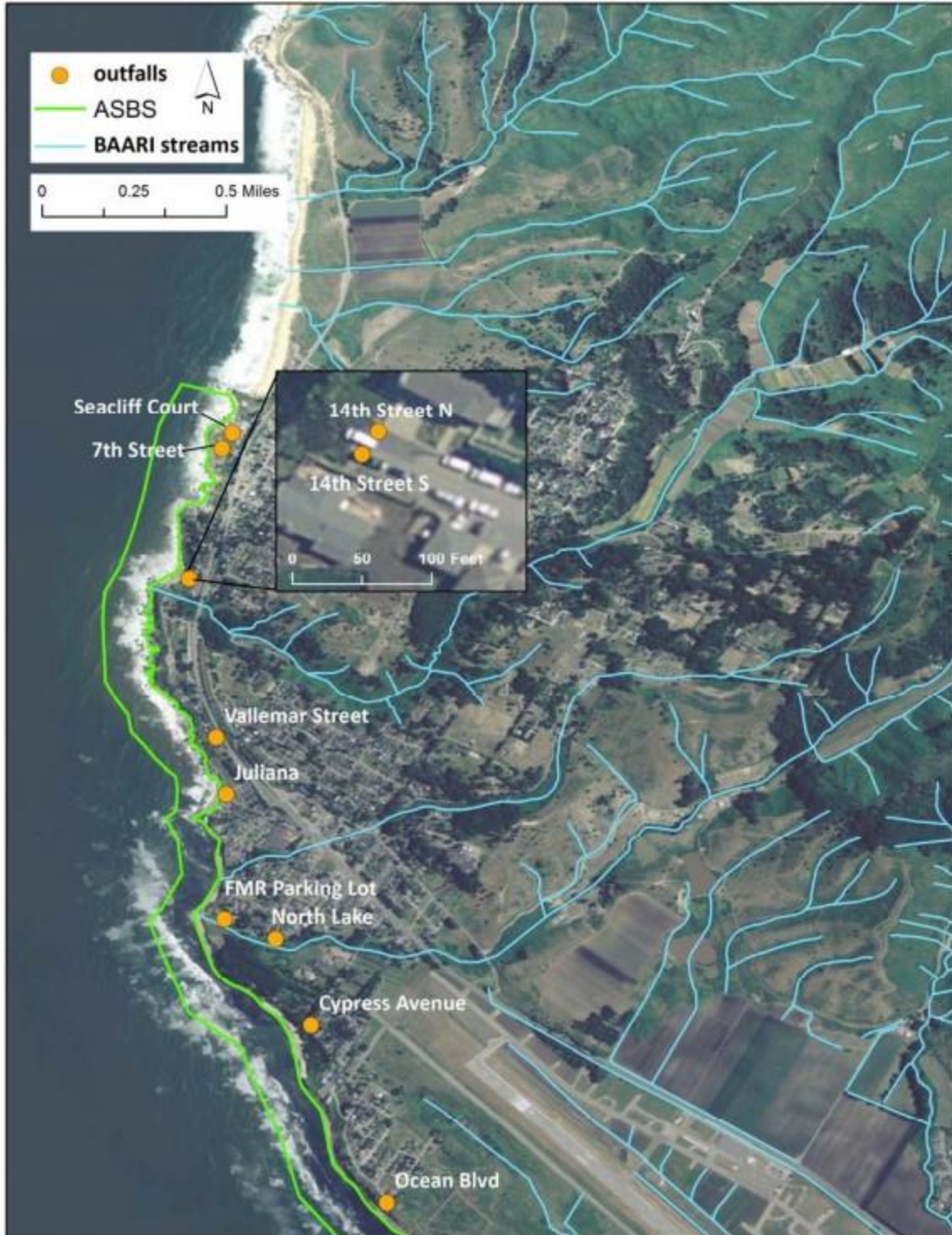
Picture 6: Map Project overlays areas with drainage outfalls to ASBS into Fitzgerald Marin Reserve, including Deans Creek, Juliana St, Vallemar St and FMR Parking Lot.
