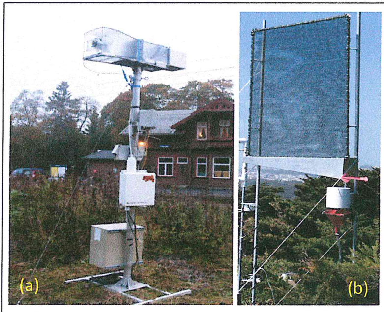
Figure 1. (a) active fog collector CASCC2, which is similar to (larger and mounted higher than) the CASCC we aim to deploy at MWSD, (b) passive mesh collector and gauge.
